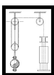
A pipe is suspended from a wire rope connected to a dead weight by using a pulley mechanism. As the pipe moves up the dead weight moves down and moves up when the pipe moves down. The weight of the pipe is perfectly counterbalanced by the dead weight such that the pipe can be said to be floating, the supporting force remains constant irrespective of movement.
