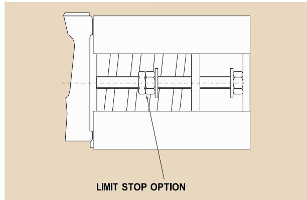
2. The supports can be supplied with plastic coated coils for superior corrosion resistant properties. The partnering spring can and attachments need to be Hot dip Galvanized. Since the support is of a bolted construction no welding activity takes place after galvanizing
