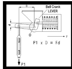
The Bell crank lever rotates around the Fulcrum point 'O'. One end of the Bell crank lever is connected to the pipe 'P1', the other end is connected to the spring by the tie rod. Thus when the pipe moves down from cold to hot condition, the point P1 moves down, and as it moves down the Bell crank lever will rotate in the anti clock wise direction & tie rod connected to the spring will be pulled in, by which the spring gets further compressed.
