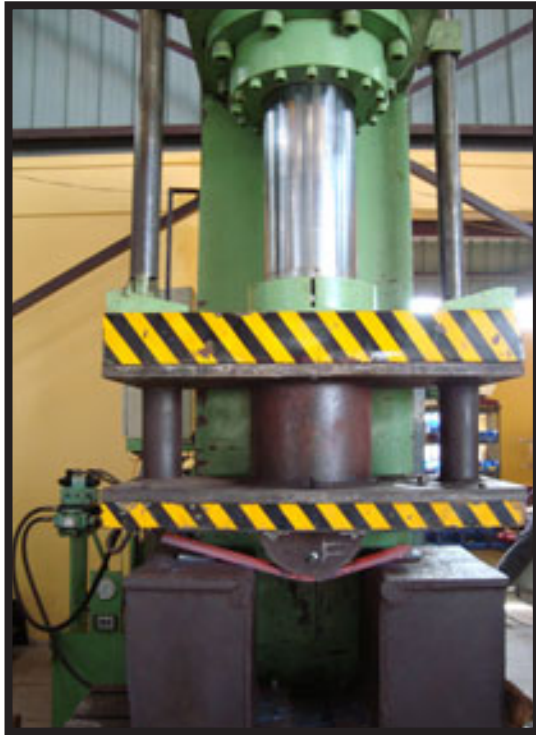
Clamps being hot formed in 150T press
